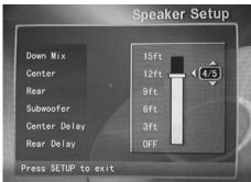
Figure 7. Establishing Center and Rear Speaker Delays
